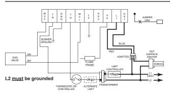
Fig. 1 – Typical hookup for White-Rodgers replacement with indirect sense using flame probe
